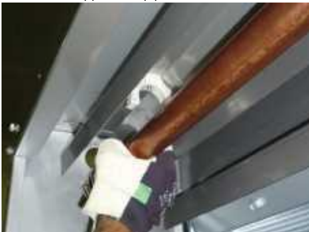
Release copper collector from plastic holders
